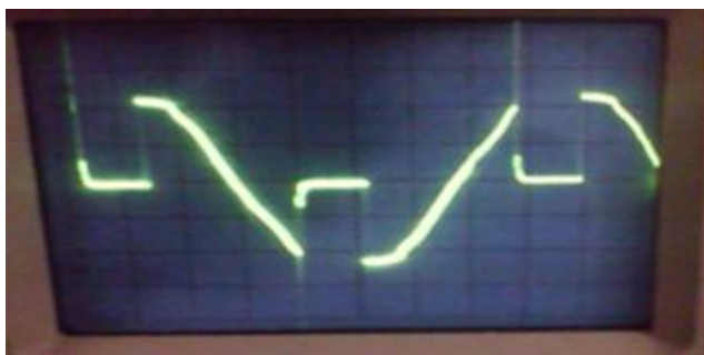
Fig.14. Wave form across inductance when \alpha = 85^\circ
