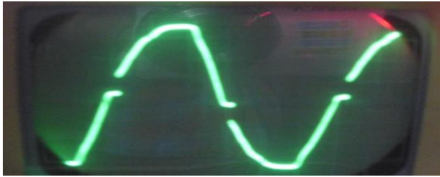
Fig.10. Wave form across resistance when \alpha = 18^\circ
