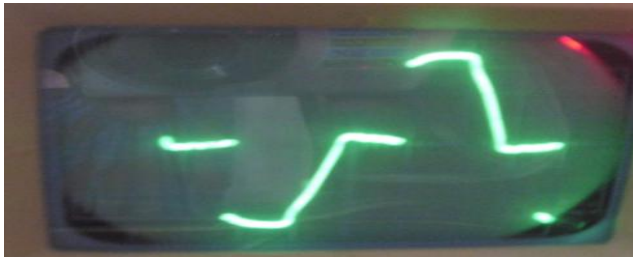
Fig.11. Wave form across resistance when \alpha = 58^\circ
