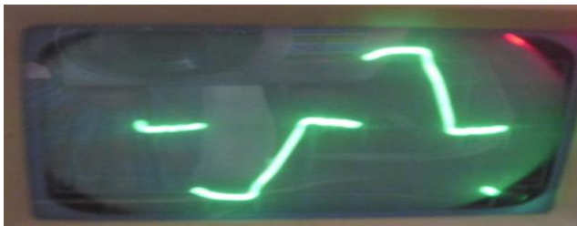
Fig.12. Wave form across resistance when \alpha = 90^\circ
